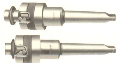
Views show action of the latches as the collet is raised into the chuck.
